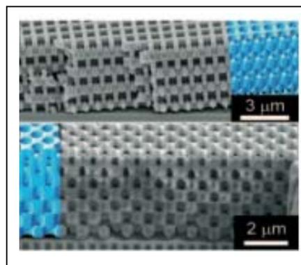
**Figure 2:** Inorganic 3D photonic crystal created via interference lithography.
