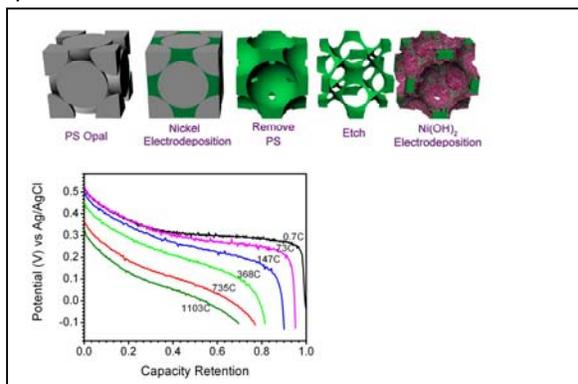
**Figure 1:** Top, fabrication process for forming the battery electrode. Bottom, discharge characteristics as a function of discharge rate (1C = 1 hour discharge).
