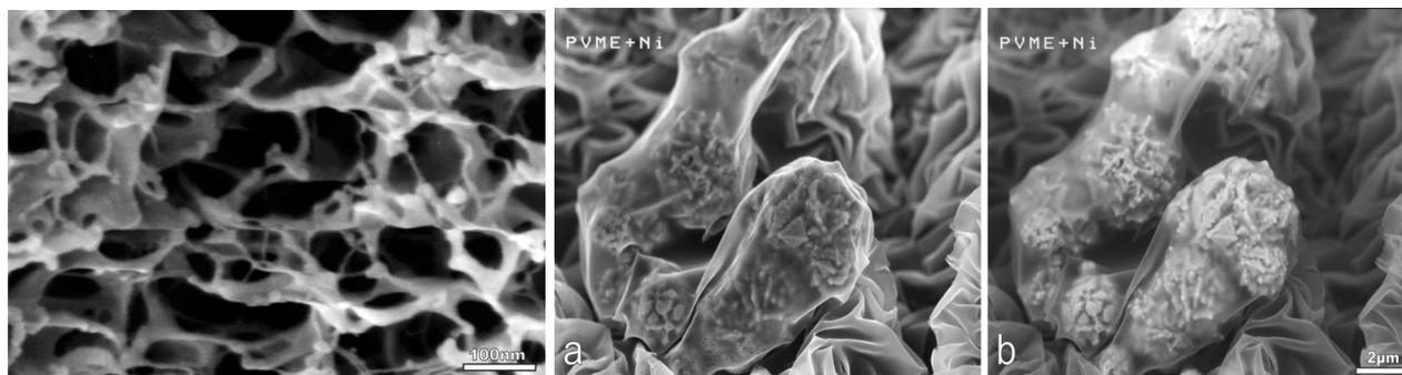
**Figure 1:** PNIPAAm hydrogel imaged in FESEM with SE. The bar corresponds to 100 nm.
