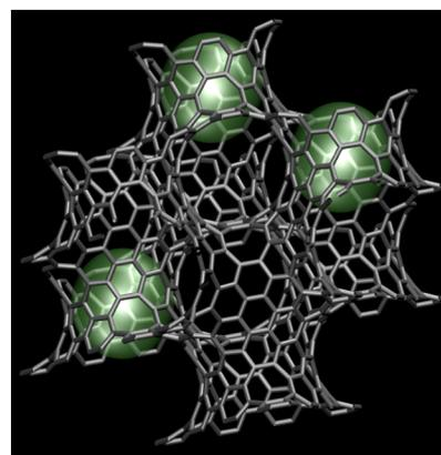
Unit cell of a typical carbon nanonetwork, representing a junction between multiple carbon nanotubes. This system possess interesting transport properties and can be tailored into a useful device. It is also a model system to study nanoporous carbon for electric energy storage applications.
