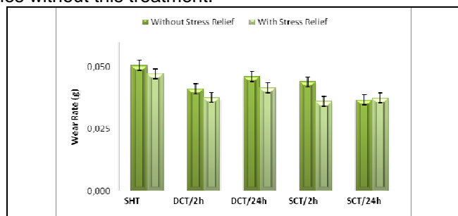
Figure 2 – Wear rate of the samples with and without stress relief previous to the cryogenic treatment.
