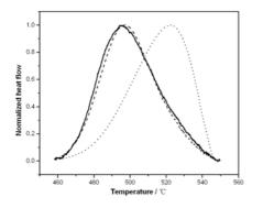
**Figure 1:** Theoretical and experimental DSC curves at heating rate of  $5^{\circ}$ C/ min. Experimental curve (solid line); JMA theoretical curve using constant activation energy and Avrami exponent (dotted line); JMA theoretical curve using variable activation energies and Avrami exponents (dash line).
