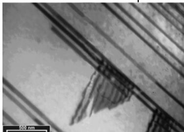
Figure 2: TEM image of 30Mn rolled at 20°C and annealed at 1000°C: dislocations are removed. Some martensite plates and stacking faults are observed in broad grains.
