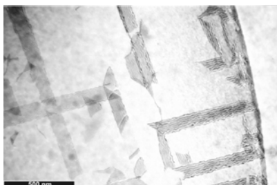
Figure 5: TEM image of the 15Mn alloy, unidirectionally rolled at 800°C and annealed at 600°C. It shows stacking faults aligned in two directions.
