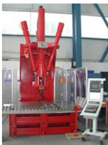
Figure 1 – FSW Tricept Robot 805 and Siemens Sinumeric 840D controller
