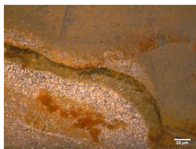
Figure 2: – Surface optic micrograph displaying corrosion after immersion.
