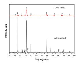
**Figure 1** XRD diffraction patterns of the as-received commercial  $MgH_2$  powders and of the compacts produced by cold rolling. In the cold rolled sample, a small amount of the metastable γ-MgH<sub>2</sub> phase is present. The β-MgH<sub>2</sub> hydride is highly oriented accordingly to (101) and presents a crystalline grain size of 20 nm, as estimated by Scherrer analysis.
