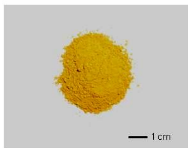
Figure 1: Photograph of the obtained CdS powder.
