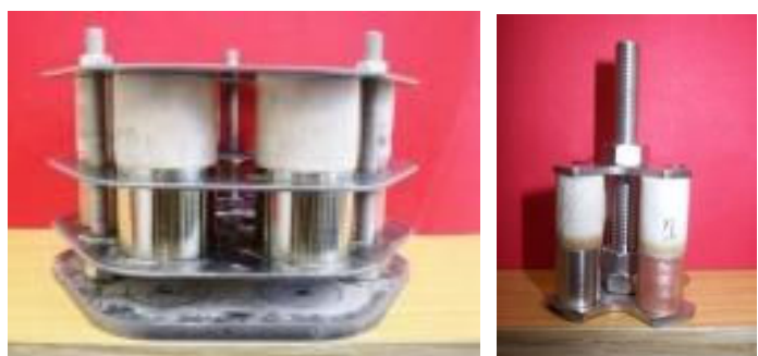
Figure 2: a) Support used for brazing of samples of \text{Al}_2\text{O}_3 and \text{SiC} with steel and copper. b) Support of the samples used for brazing of \text{ZrO}_2 with steel and copper.
