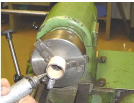
Figure 1: Process of mechanical metallization
