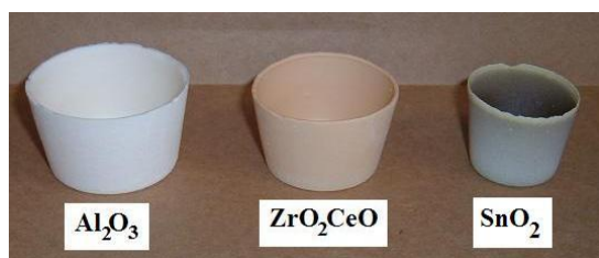
Figure 1: High-density homemade crucibles of Al_2O_3 , ZrO_2CeO and SnO_2
