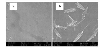
Figure 3: SEM of ZnO films a) undoped ZnO; b) ZnO:15at%Ca.
