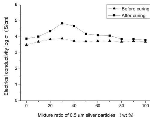
**Figure 2:** The electrical conductivity of silver paste films using two different diameters of silver particles and MTAZ, before and after curing at 80 °C for 6 h.
