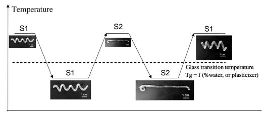
Thermomechanical process of shape programming / recovery of extruded potato starch
