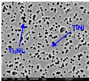
**Figure 1:** SEM image of the characteristic microstructure of type N alloy.
