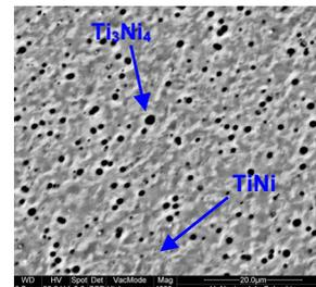
**Figure 2:** SEM Image of type N alloy after heat treatment was carried out.
