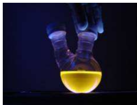
Figure 2: Fluorescent CdSe/CdS core-shell quantum dots in aqueous medium. (Excitation wavelength = 365nm).
