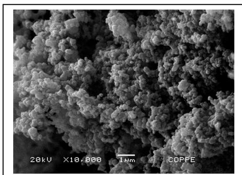
Figure 1: SEM image of nanospheres obtained at 1000°C.
