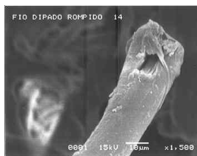
Figure 3: Multi axial stress fracture of the heat-treated monofilament
