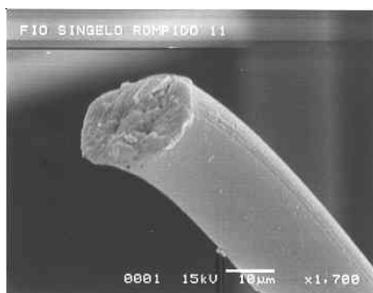
Figure 1: Ductile fracture of the regular monofilament
