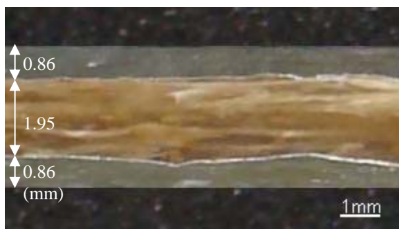
Figure 1: Cross-sectional view of the hybrid composite showing the three layers (glass/sisal/glass).
