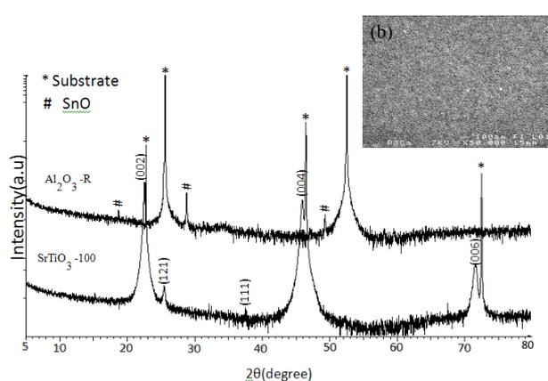
**Figure 2** –  $\text{CaSnO}_3$  thin films treated at 700° C for 2 h: (a) XRD patterns (b) SEM images
