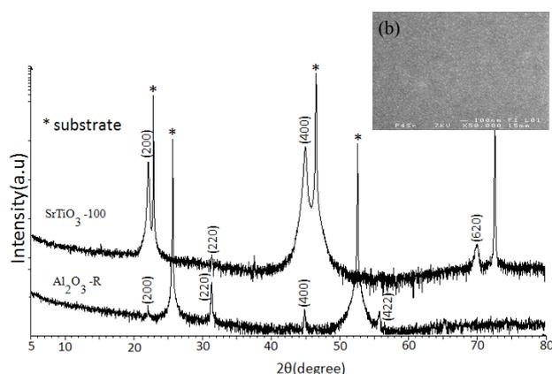
**Figure 1** –  $\text{SrSnO}_3$  thin films treated at 600° C for 2 h: (a) XRD patterns (b) SEM images
