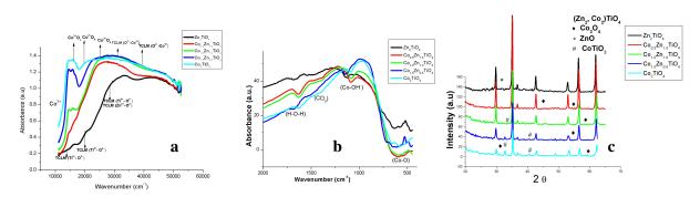
Figure 1: (a) IR spectra, (b) UV-vis spectra and (c) XRD patterns of the  $Zn_{2-x}Co_xTiO_4$  ( $0 \le x \le 2$ ) calcined at 800°C.
