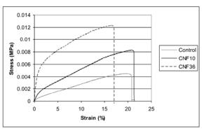
**Figure 1:** Stress-strain curves for MPEF with CNF loadings of 0% (control), 10% (CNF10), 36% (CNF 36).
