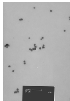
Figure 2: TEM of 42 nm Silica nanospheres
