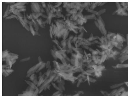
**Figure 2:** FEG-SEM micrographs of  $\text{MnWO}_4$  powers processed in hydrothermal-microwave at 413 K for different.
