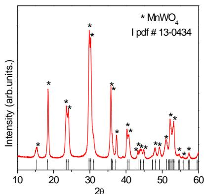
**Figure 1:** XRD patterns prepared by the hydrothermal-microwave of  $\text{MnWO}_4$  15 min.
