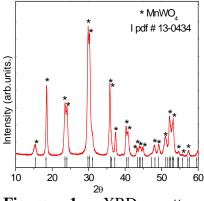
**Figure 1:** XRD patterns prepared by the hydrothermalmicrowave of MnWO<sub>4</sub> 15 min.
