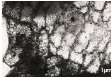
Figure 1. Sub-grain structure of polygonized aluminum.
