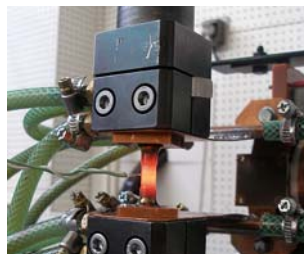
Figure 2: TMT of AHSS 42SiCr with integrated Q-P process
